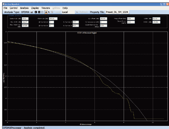
Figure 9. The CCDF plot is a versatile method of evaluating WiMAX transmitter and power amplifier nonlinear behavior.
