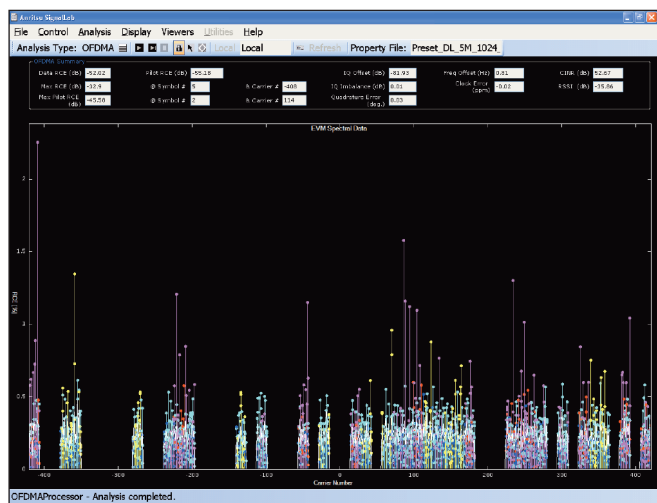
Figure 7. Error vector magnitude (EVM) is a powerful tool for evaluating the modulation quality of a WiMAX transmitter. Here is shown as an EVM spectrum.
